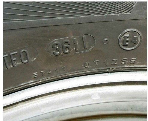
The date code shows when the tyre was manufactured
