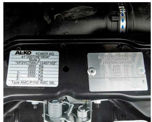
Weight plates - the original vehicle manufacturer's plate left and the AL-KO plate (or convertor's plate), which supersedes the original plate, on the right
