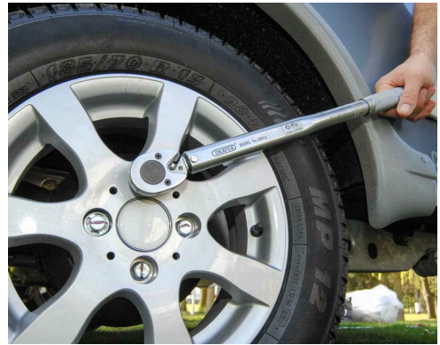
Check wheel nuts with a torque wrench
